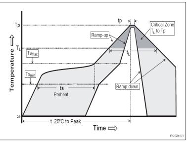
Note that this product will be easily damaged by rapid heating, rapid cooling or local heating.
